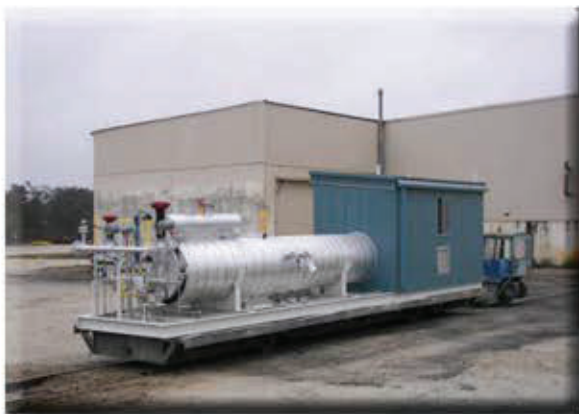
Chemical Dosing Skid
