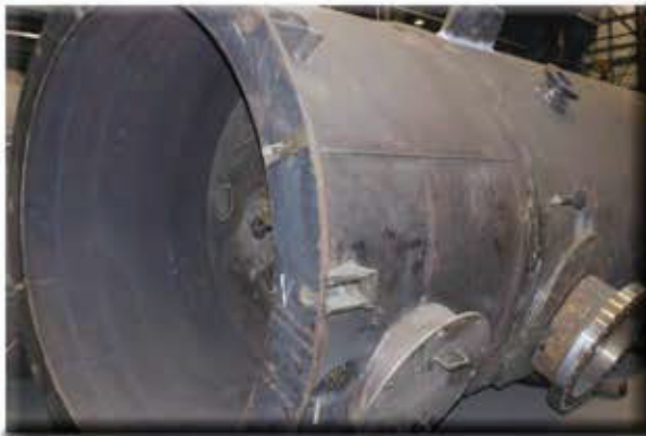
Heavy Wall Pressure Vessel
